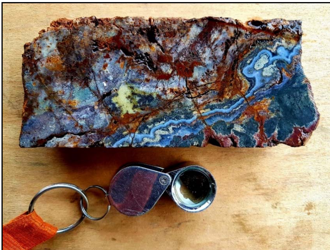
Classic banded epithermal vein from an interval in CZDD001 that assayed 342 g/t Ag (89.0m to 89.8m). Silver assay results are very similar to results from historic drilling.
