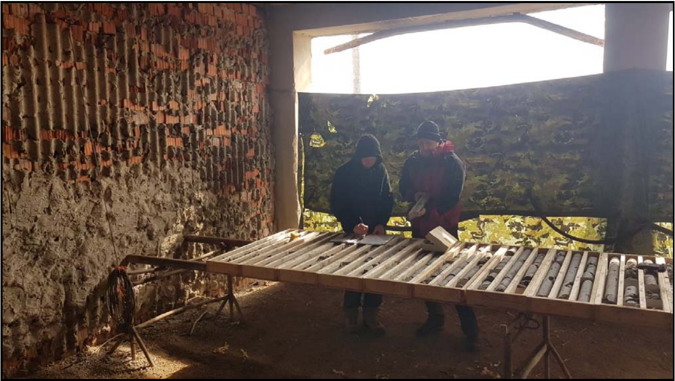
Onsite processing of core at Zemplin before dispatch to processing facilities.
