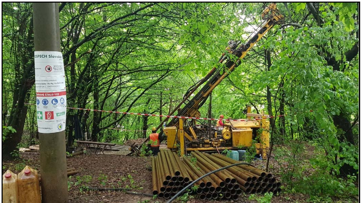
Diamond drill rig set up and drilling the first Krakauer hole, KVDD001.
