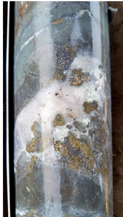
Core from CZDD006 at 130m showing polymetallic (silver, lead, zinc) epithermal mineralisation.
