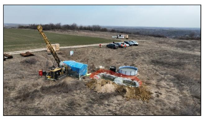
Set up on CZDD005 which was designed to test the strike and depth potential of a fully preserved silver and base metal mineralised system.
