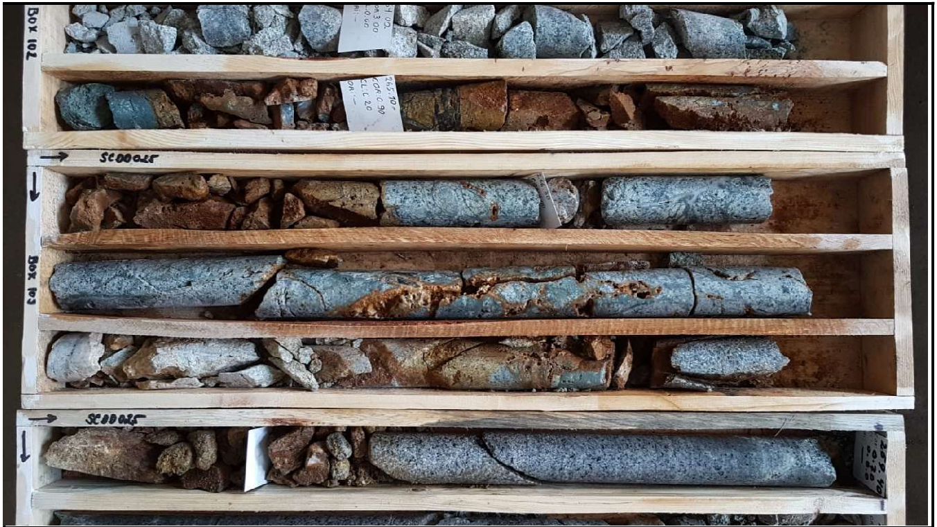
Quartz veinlets with minor base metal sulphides at 265m - 268m in SCDD025.
